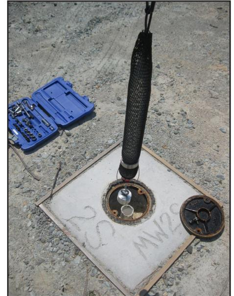
*The passive diffusion bag technique is used on environmental restoration sites at Fort Bragg, North Carolina, as a less invasive option for sampling groundwater. Once the bag is deployed, it is removed and tested for volatile organic compounds. (U.S. Army photo)*
